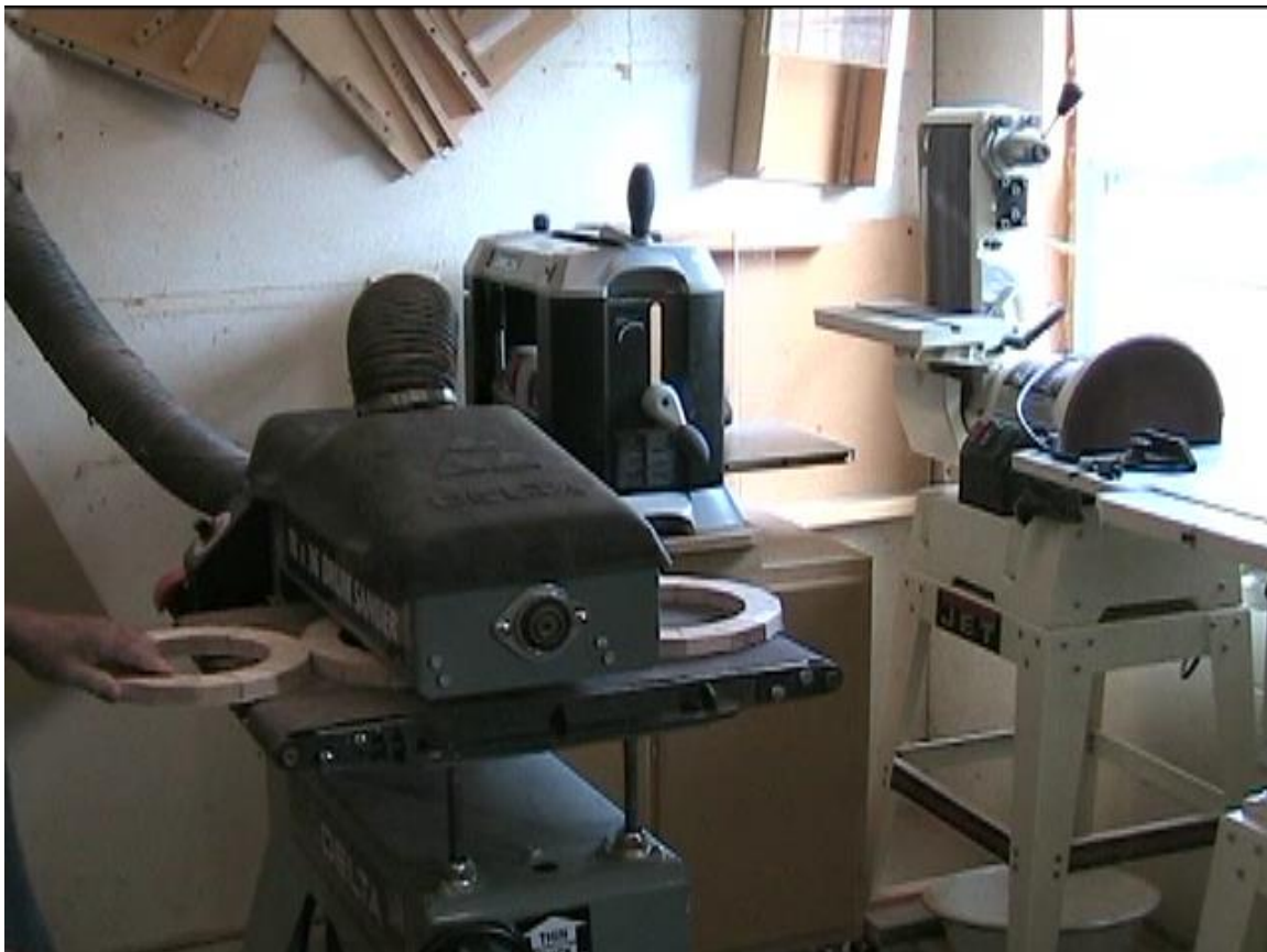
Figure 12. Using Drum Sander to flatten the rings after assembly.
