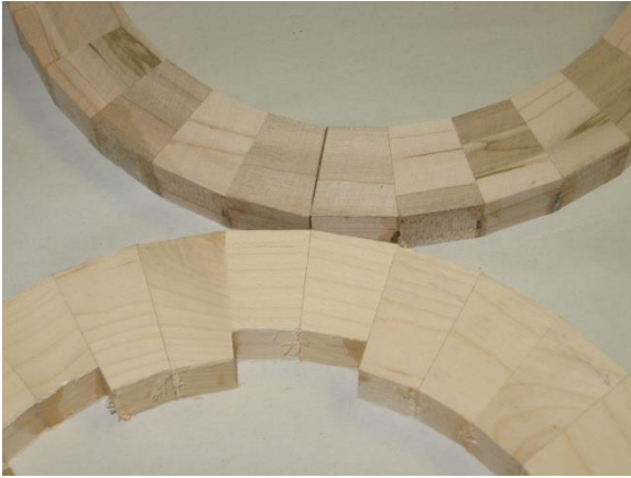
Figure 4. Comparison of doctored joint and good one
