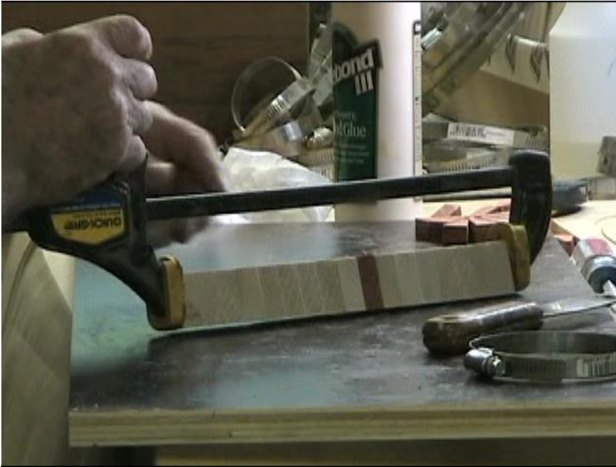
Figure 10. Shortcut for gluing. Segments are aligned and clamped so that glue can be applied to all needed surfaces.
