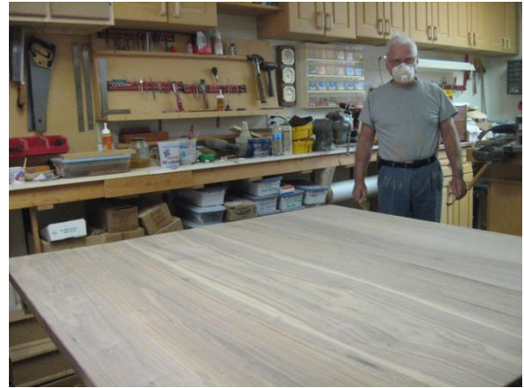
Figure 14 Sheet sanding completed.
