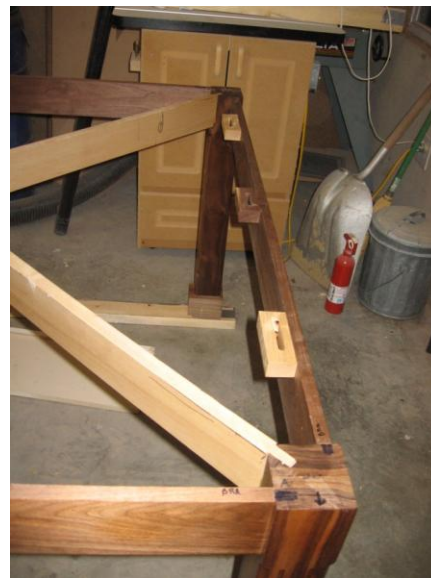
Figure 17 Hold downs for the table top. Screws were centered in the slot and driven into the table top thus allowing movement in the cross grain direction.
