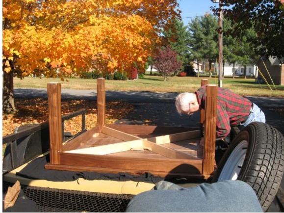
Figure 18 Attaching undercarriage to upside down table top.
