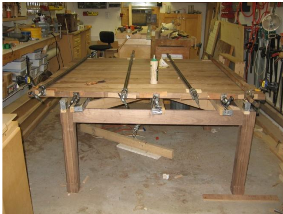
Figure 12 Final glue up of top. Note use of 7 clamps
