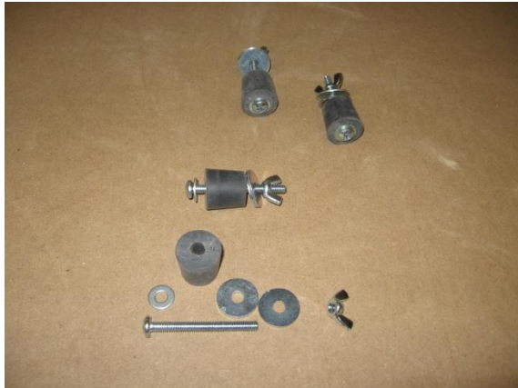
Figure 7 Gripper assembly with stopper; 1/4" screw; wing nuts; fender washers; and 1/4" flat washer
