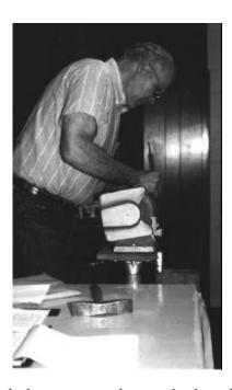
Here Bob demonstrates how to look at the sparks given off by a piece of metal on a grinding wheel.
