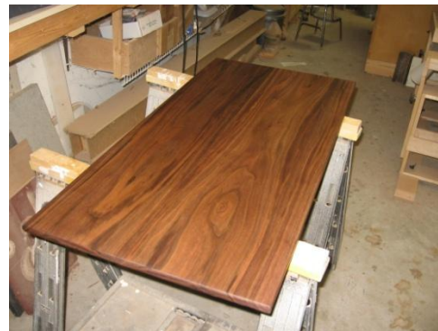
Figure 21 Table top after one application of oil slurry filling the pores in the grain.
