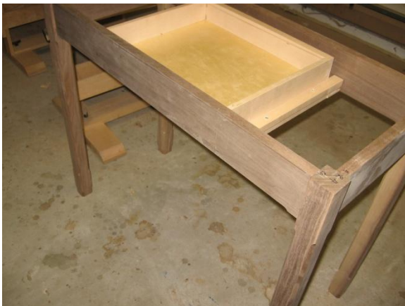
Figure 17 Drawer fitted into frame and flush with front apron.
