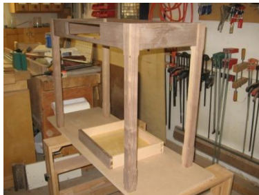
Figure 13 Glued together aprons and legs.
