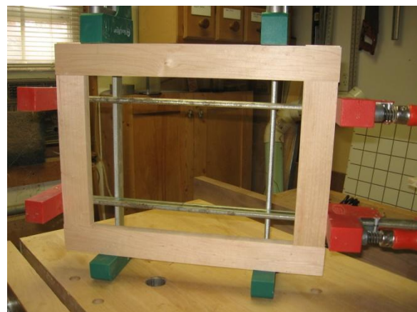
Figure 12 Bessey Clamps used to keep frame squared during glue up
