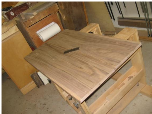
Figure 7 Table top with scraper used to level joint of the two boards
