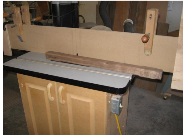
Figure 8 Jig used on router table to chamfer table legs
