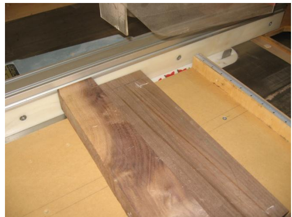
Figure 5 Setup for making grooves around all apron ends in preparation for making tenons
