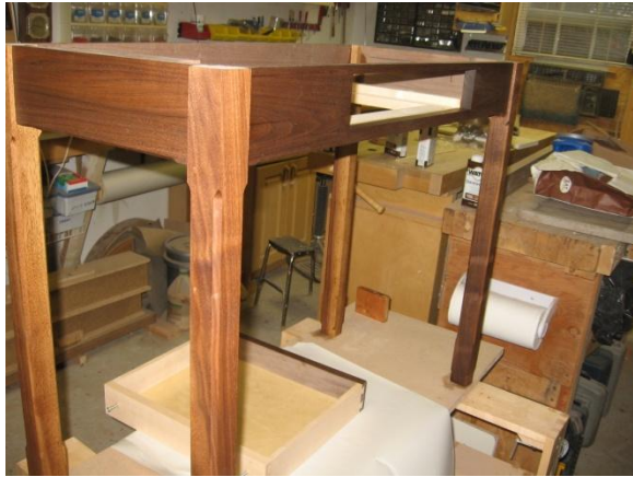
Figure 22 The base assembly after treatment with dark Watco wiping varnish
