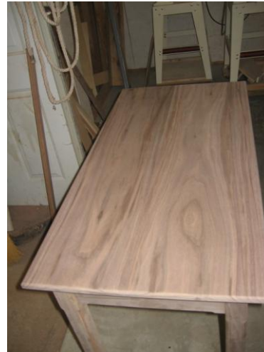
Figure 20 Table top prior to filling the grain with oil slurry.
