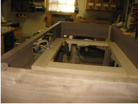
Figure 16 Orientation of frame in table during attachment process. Note how frame is held flush with bottom edge of drawer opening.
