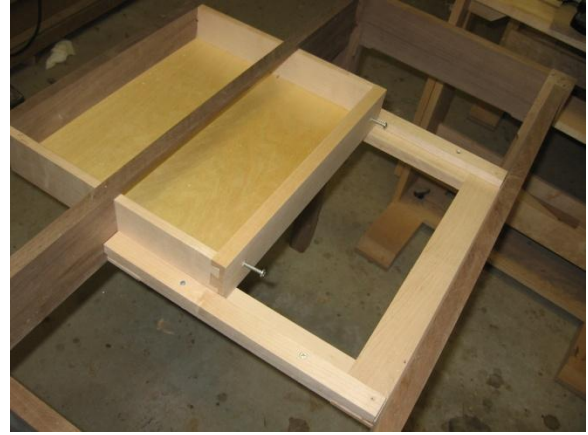
Figure 18 Drawer partially closed revealing depth adjustment screws. The screws ride with the drawer so that depth adjustment can be easily accomplished.
