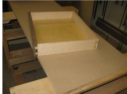
Figure 14 Drawer glued up. Note half blind dovetails front and back
